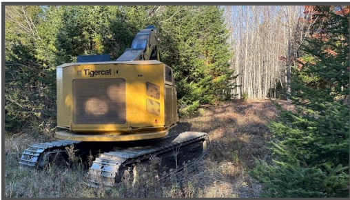
A timber harvester positioned at an entry point to the forest. 12 - 15 foot pathways were cut to access the site.
